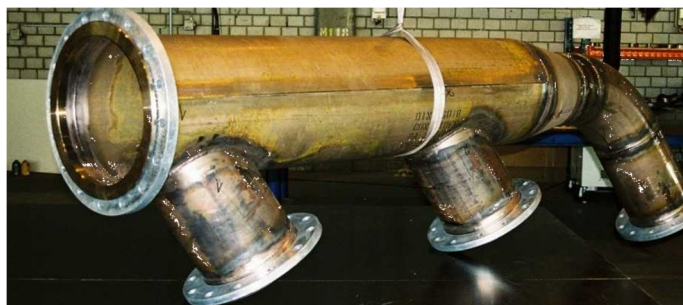
CuNiFe manifold, assembled, fire fighting system
