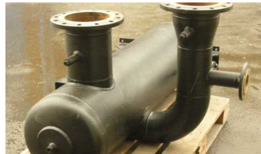
Carbon Steel, steam, 14 bar, PED
